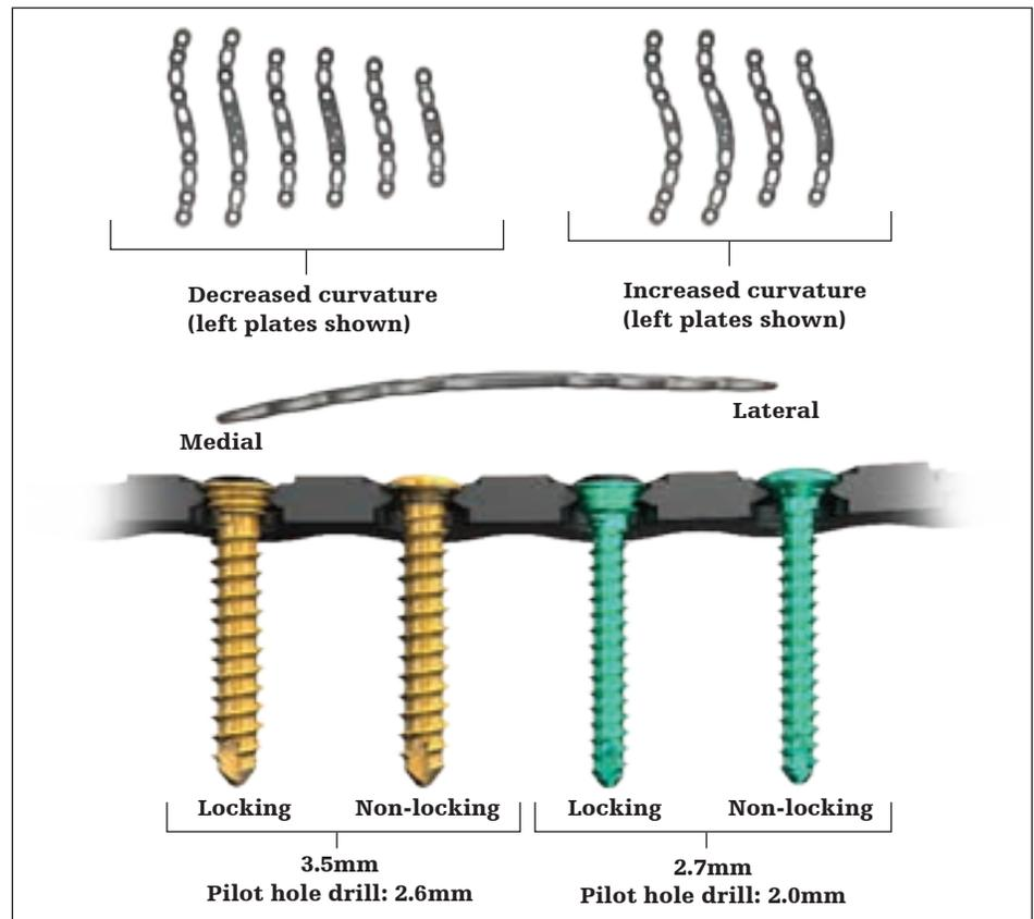
**Note: Only non-locking screws may be placed in the oblong holes of the plate. Circular holes accept either locking or non-locking screws.**
