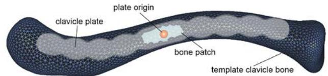
**Figure 2:** Definition of bone patch (light blue) which defines the tolerated movement of the implant on a template clavicle (red ball marks defined plate origin)
