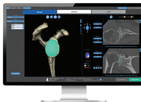
Figure 2. Main window of Blueprint for selecting the suitable position of the glenoid implant in accordance to the version, the inclination, the reaming depth and the seating.
