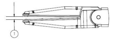
1 < 2 mm – Confirm that the jaws are in the closed position prior to activating the cutter.
