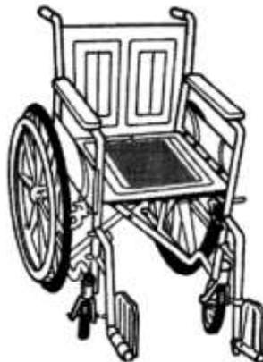
Figure 1 – Posey® Chair Alarm Sensor Pad Positioning
