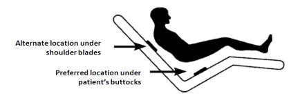
Figure 1 – STANLEY® (Securitas Healthcare) Bed Alarm Sensormat® Pad Positioning
