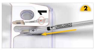
Insert the tip of the eyelet inserter into the eyelet and press to engage the eyelet with moderate pressure. A slight click may be felt at this time.
