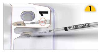
Orient the eyelet inserter handle so that is facing up and the arrow is pointed toward the eyelet. The inserter will be slightly angled, as pictured, for ease of insertion.
