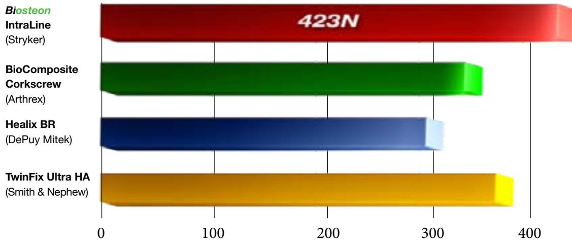
One pound force is approximately equal to 4.5 Newtons. All anchors above are 5.5mm.
