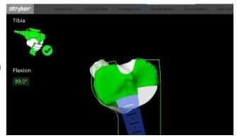
The surgeon completes bone preparation using  $AccuStop^{TM}$  haptic technology. The saw is constrained in the virtual boundary that is established by the surgeon's patient-specific plan, as seen in step 5.
