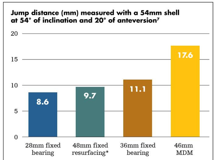
Figure 2. Jump distance comparison of MDM against fixed bearings and resurfacing shells
