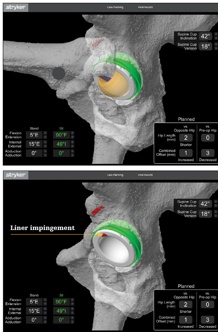
Figure 3. Mako THA has virtual range-of-motion tool indicating risk of impingement (highlighted in red). The surgeon is able to change implant position and/or implant systems to address impingement.
