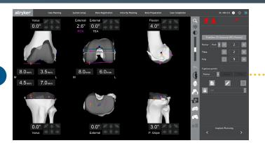
The 3D CT-based pre-plan demonstrates that the operative knee is in varus, set to the default planning parameters and planned component sizes are 2 femur and 2 tibia with the Triathlon Knee System.
