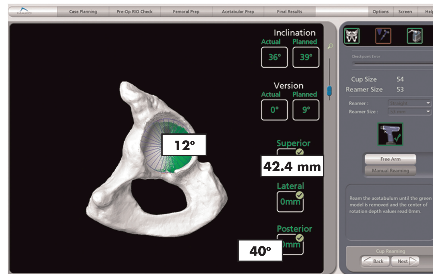
Fig. 2 Computer screen showing the completion of reaming with all COR numbers reading zero and the bone color changing from green to white. Source: MAKO Surgical Corp.
