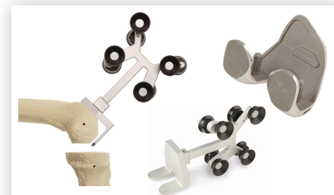
Fig. 1 Navigated probe and example measurements of bone resection (shown for anterior chamfer cut on femur). For measurements of component position, the femoral component was modified with posterior flats.
