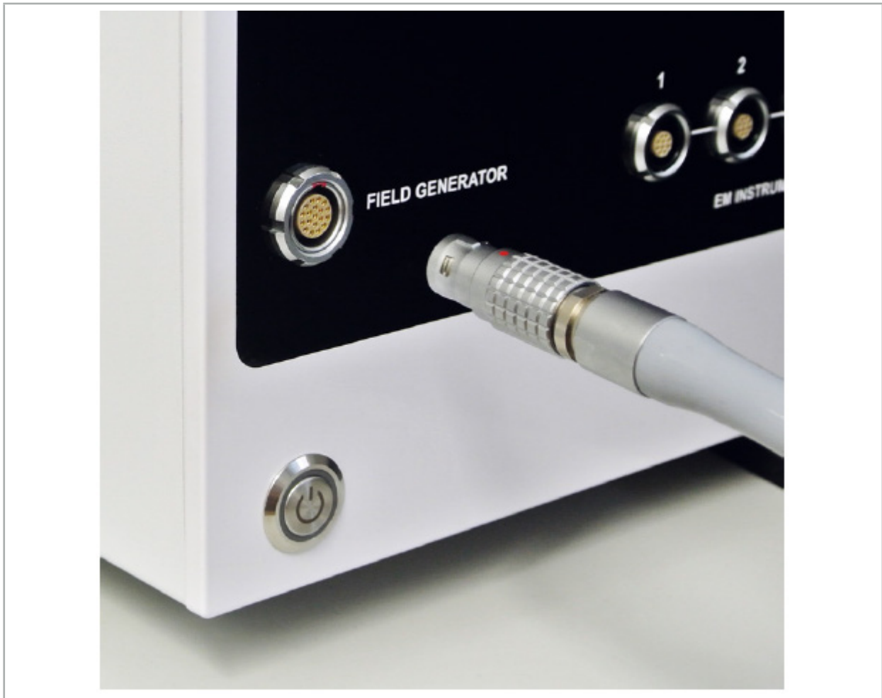
Figure 38 – Connecting the Field Generator Cable to the Navigation Unit
