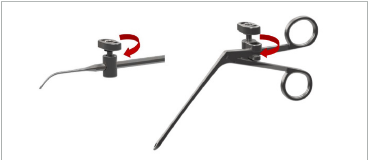
Figure 52 – Fixing the Instrument Clamp to the Surgical Instrument
