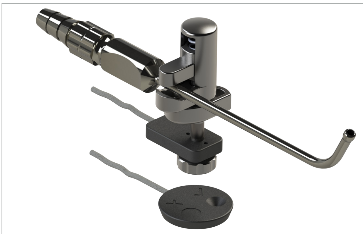
Figure 100 – Hold the tracker up-side down over patient tracker to reset calibration
