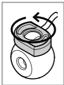
Figure 3 - Step 1: Unscrew the clamp fastening nut (counterclockwise).
