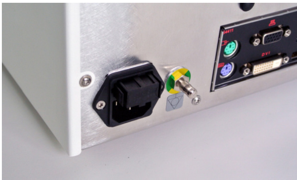
Figure 4: Opening the Fuse Box
