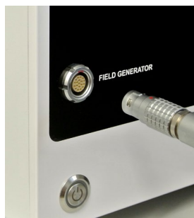
Figure 98 Connecting the field generator cable to the Electromagnetic Navigation Unit
