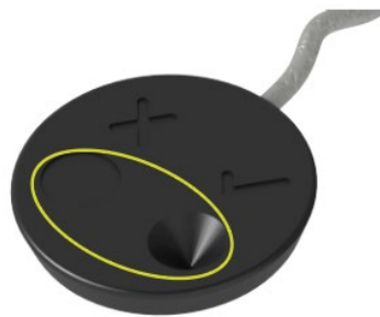
Figure 126 Calibration areas (cone and plane) exemplified on the base of the tracker
