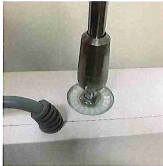
Example of Mounting Arm Threaded into Field Generator
