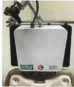
Example of Rail Clamp Attachment and Field Generator Storage Location
