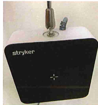
Example of Mounting Arm Threaded into Field Generator
