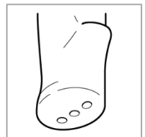
Figure 4: Cryogen gas exits from the exhaust ports on the bottom of the cryoprobe.
