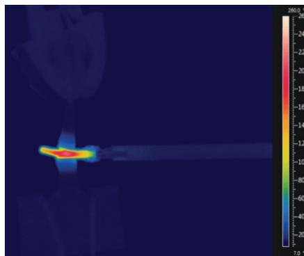
Figure 5. FLIR image of HARH jaw and shaft during porcine carotid artery transection.
