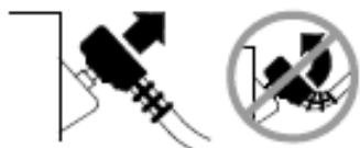
Figure 5-7 Disconnecting Defibrillation Cable from Test Post
