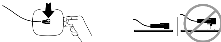
Figure 5-4 Connecting FAST-PATCH Electrodes to Defibrillation Cable
