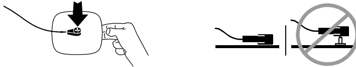
Figure 5-4 Connecting FAST-PATCH Electrodes to Defibrillation Cable
