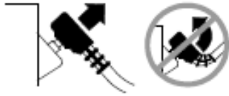
Figure 5-7 Disconnecting Defibrillation Cable from Test Post
