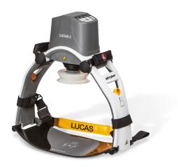
The LUCAS chest compression system includes a back plate which is positioned underneath the patient as a support for external chest compressions, an upper part which contains the compression mechanism and disposable suction cup, and the stabilization strap which helps secure the position of the device on the patient.
