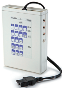
Patient simulator (QUIK-COMBO) Connects directly to your LIFEPAK defibrillator for interactive training. Select from 17 ECG rhythms including: fibrillation, tachycardias and bradycardias. 3-lead 11996-000310
