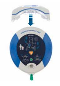
3. Slide HeartSine Gateway onto the top of the AED allowing the four pins to connect with the contacts on the data port of the AED. When HeartSine Gateway is fully connected, an audible click should be heard as the locking clips snap into place.
