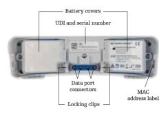
**Battery covers:** Remove to insert or replace the hatteries
