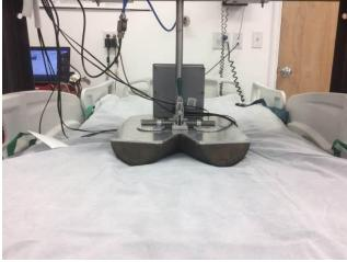
Results showed that average temperatures were comparable for all configurations, ranging from 33.4°C to 33.9°C.<sup>10</sup> Maximum relative humidity averages for configurations with a microclimate body pad were between 77.1% and 78.9%.<sup>10</sup>
