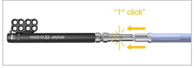
Ensure that you practice sliding the locking sleeve forward before the operation to verify that the connection is correct.
