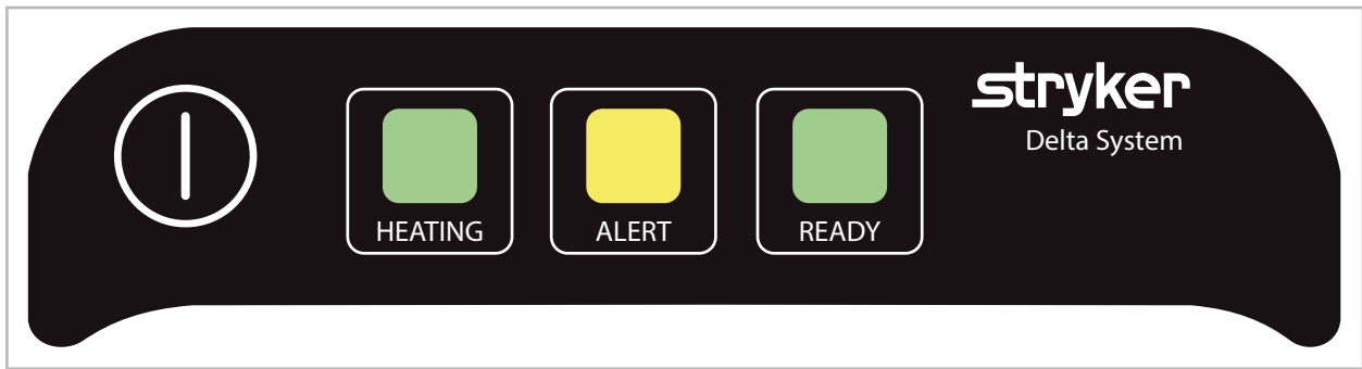
Graphic 6: Main power button and HEATING , ALERT and READY lights
