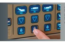
Any or all patient controls can be locked to restrict use with the patient lockout buttons. Behavioral health beds are equipped with an additional security code lock-out.
