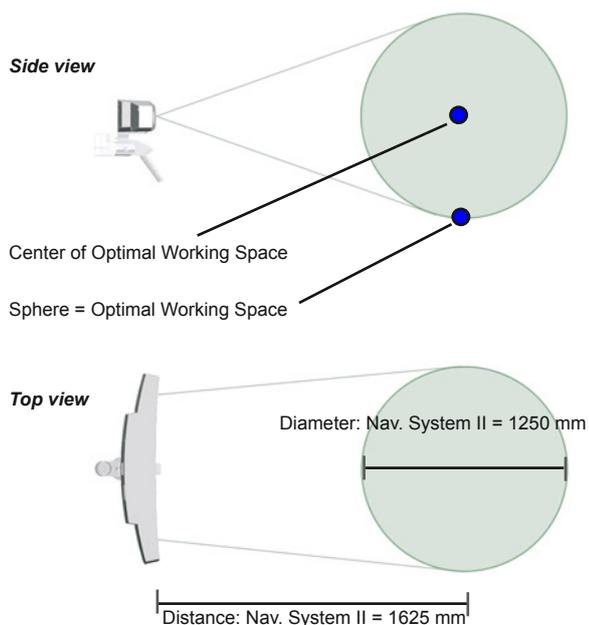
Figure 1: Navigation System Camera Working Space
