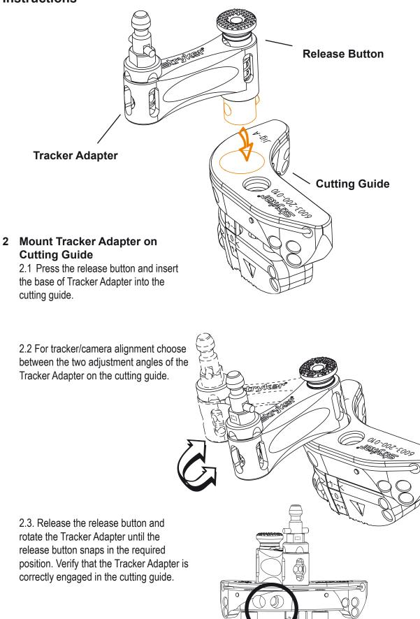
2.4 Double check that the Tracker Adapter is engaged and secure.
