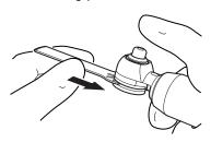
Fully depress the button and seat the blade against the post. Release the button.
