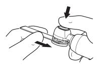
Rotate the blade against the post until it snaps into the desired location. If necessary, depress the button again to reposition the blade.
