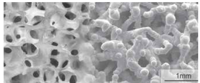
Figure 7: Cancellous bone (left) and the porous matrix of Tritanium technology (right)
