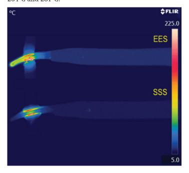
Image from time matched cut/seal sequences on <5mm vessel during benchtop testing utilizing FLIR A655sc IR camera and MARLAB script.
